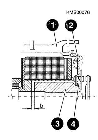
CHECKING AND REPAIRING COMPONENTS Checking return force of helical spring on engaging shaft This is performed with startingmotor assembled. It must be possible to push pinion back into rest position with spring action via rubber buffer in thrust piece of starting-motor solenoid. Engaging shaft must be seated on ball (1) in starting-motor solenoid in rest position.
